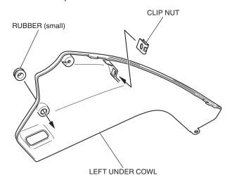
9. Install the clip nut and rubber as shown.
