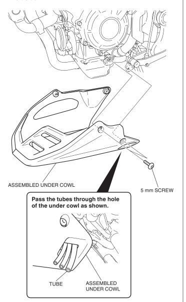
14. Loosely install the screws as shown.
