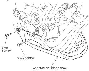
15. Tighten the screws as shown.
